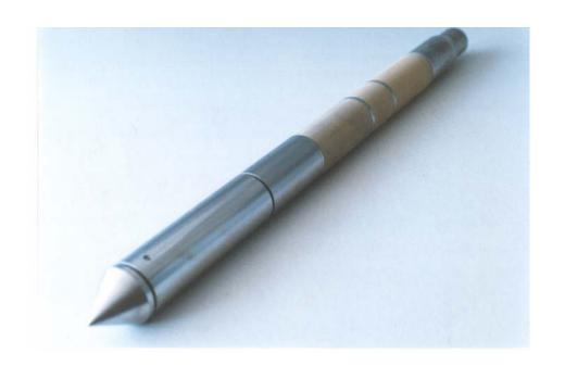
The probe measures various parameters from which the soil moisture content can be derived.
