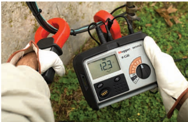
Model DET4TCR2 shown performing the stakeless ground testing method using only clamps.
