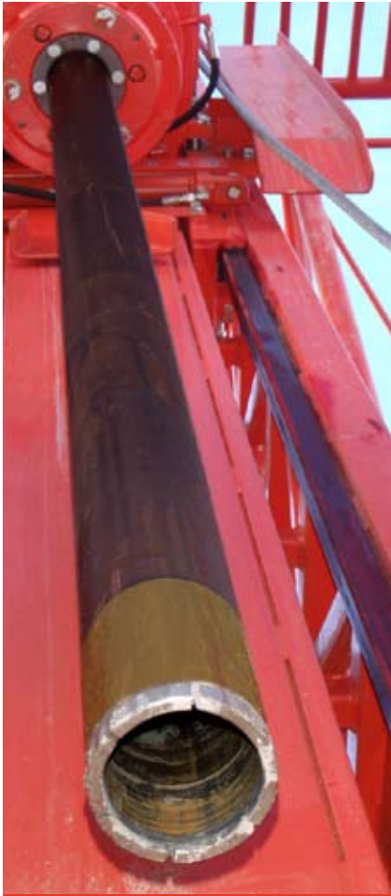
Field proven casing in operation with the DE710 surface core drill
